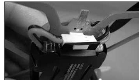
Install the flight battery from the back of the quad. Plug the battery in, paying careful attention to the plug orientation. Position the plug as shown in the picture or else unwanted vibration or flight conditions may occur.
