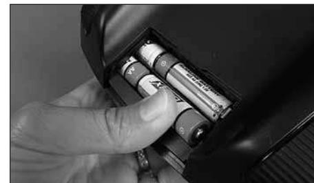
Remove the transmitter's back cover and install 4 AA batteries into the battery holder, following the battery diagram located inside the battery tray.
