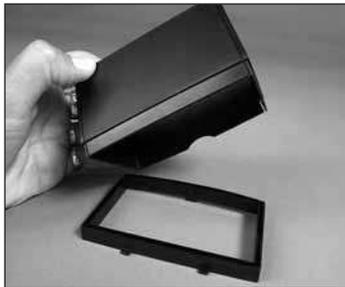
Snap the completed sun shield onto the transmitter by placing the two lower lugs into the two lower mounting holes of the screen. Rotate and snap the top lug into the upper hole to complete the assembly.
