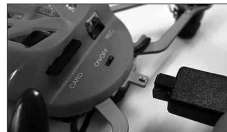
Plug the charge cable into any PC based USB port or USB adaptor.
