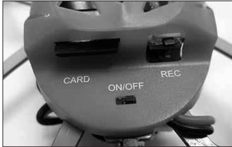
**NOTE:** Your Proto-X FPV is designed with a Power-On safety feature. This ensures that the motors will not start unless it detects a suitable control signal when the battery is connected. Make sure the throttle stick is in the full down position.
